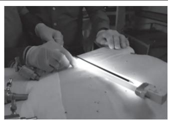
Fig. 12: Glowing of bulb due to capacitative coupling from monopolar hook
