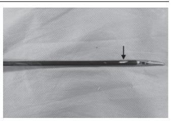
Fig. 9: Break in the insulation of monopolar scissor
