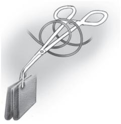
Fig. 13: Capacitance due to wrapping of monopolar code around artery forceps
