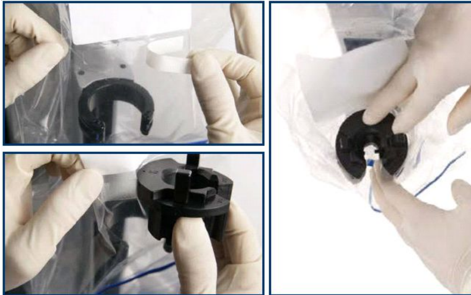
Fig. 15: Removing the Adhesive Strip and Attaching the Camera Arm Sterile Adapter
