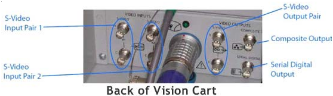
Fig. 10: Vision Cart Auxiliary Video Connectors
