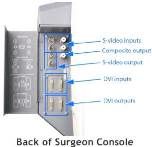
Fig. 9: Video connections on surgeon console
