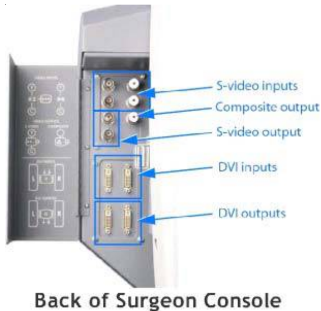
Fig. 9: Video connections on surgeon console
