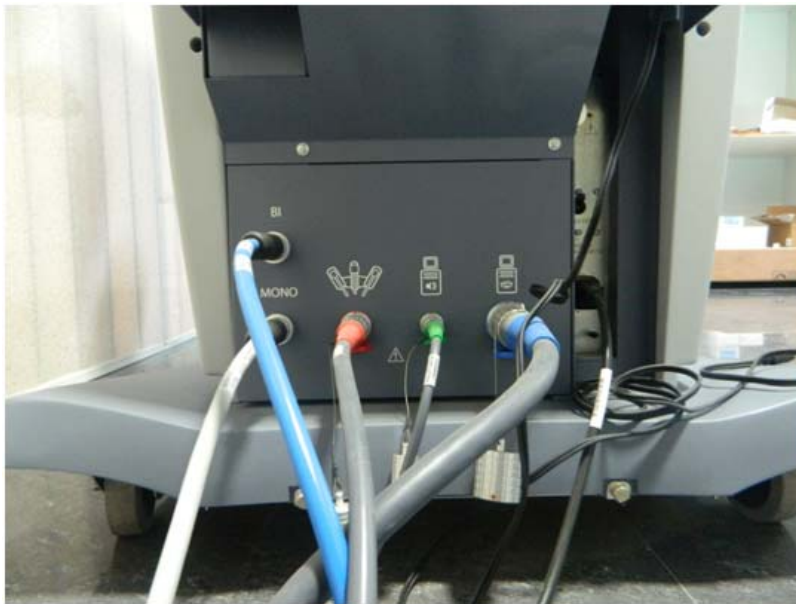
Fig. 8: Back of surgeon console with MONO and BI receptacles
