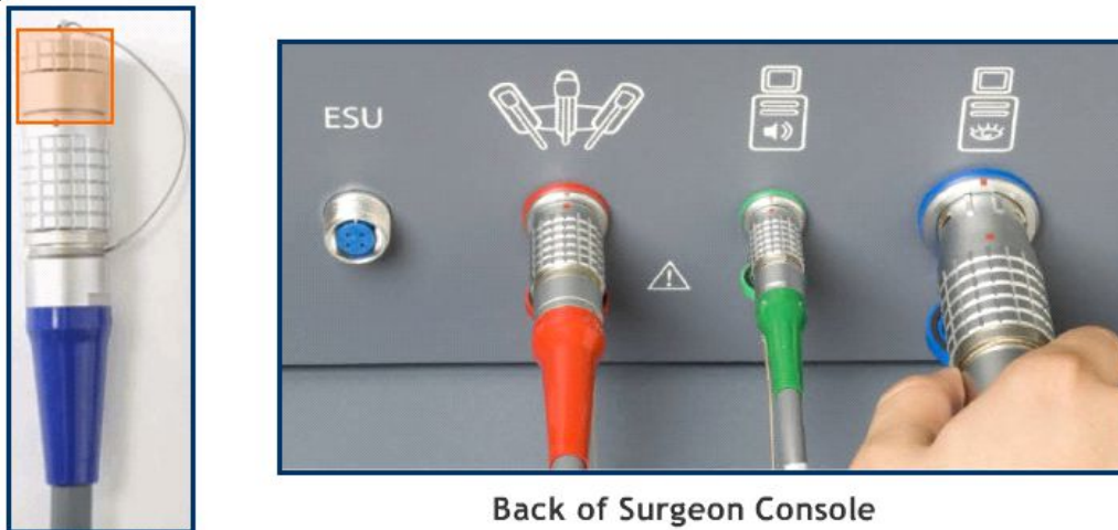
Fig. 5: Correct way of insertion of cable matching the red dot. Inset highlighting the protective cap of the cable
