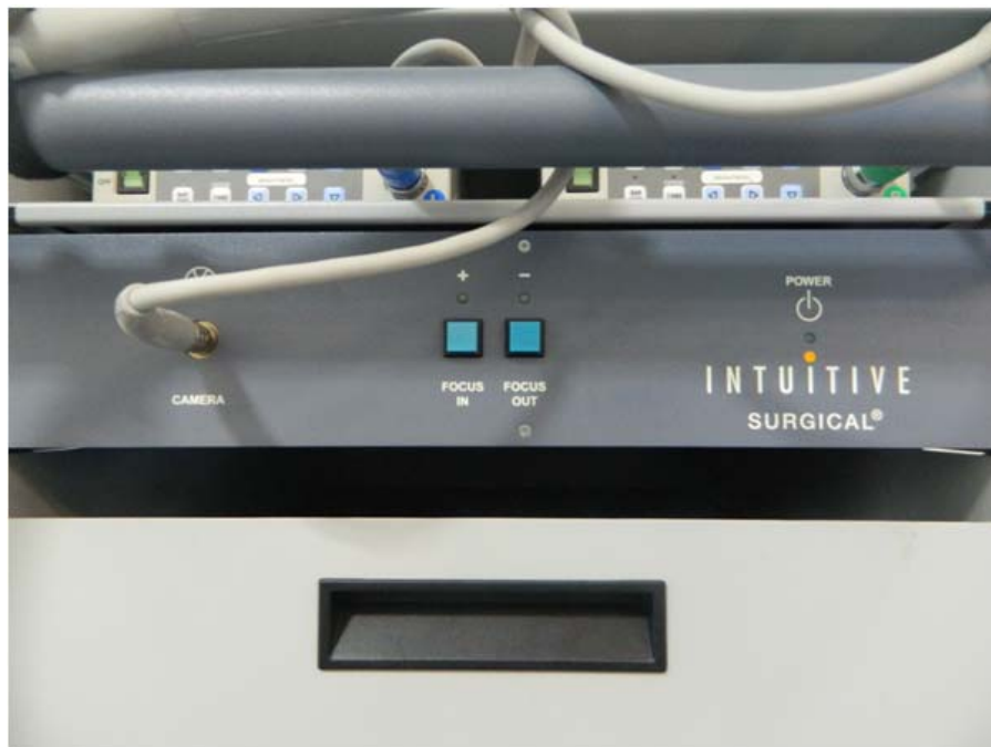
Fig. 6: Camera head cable connections
