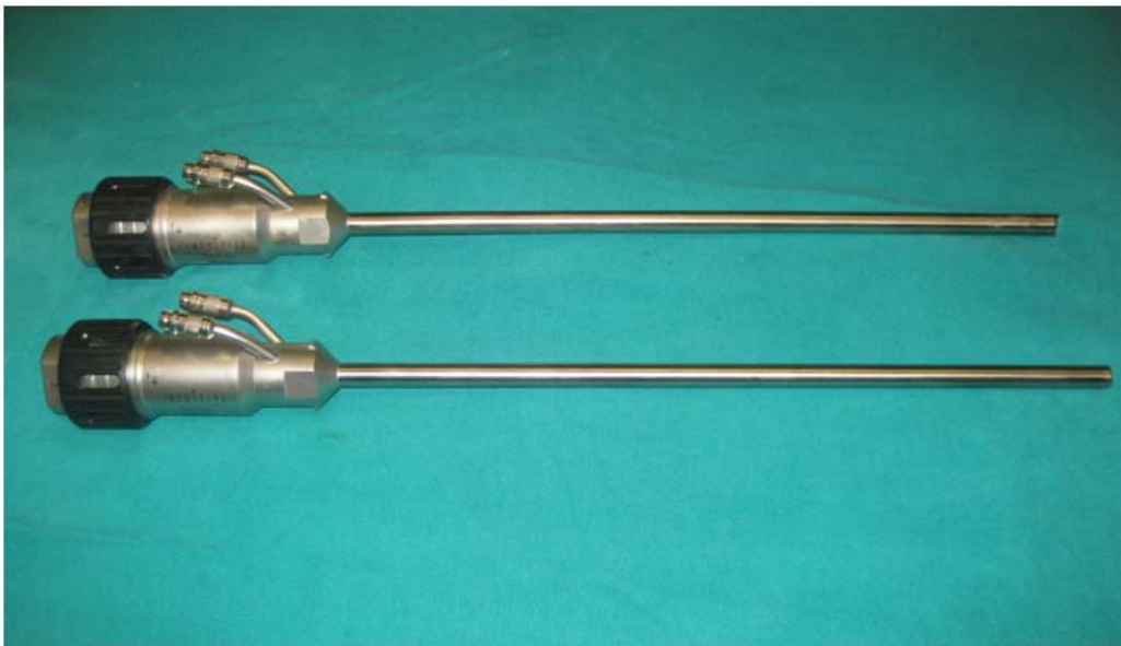
Fig. 17A: Example of 12mm 3D (30° and 0°) endoscopes
