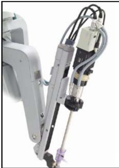
Fig. 11: Example of a Camera Arm with Attached Endoscope
