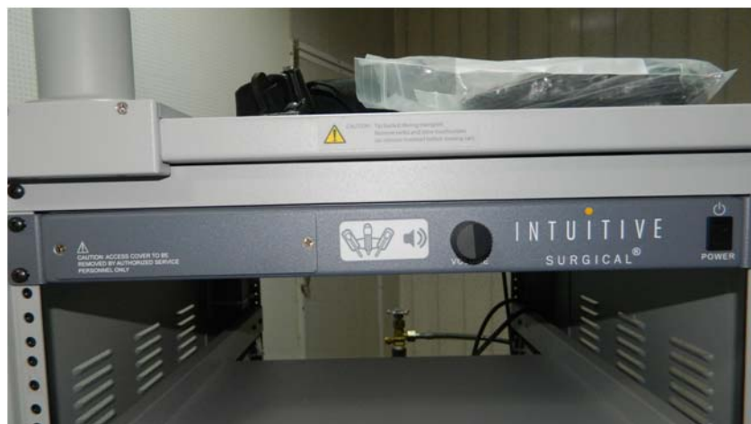
Fig. 22: Audio intercom system on top of vision cart
