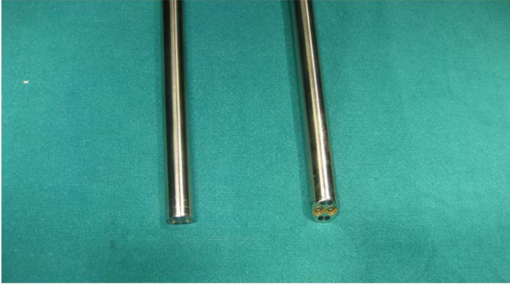
Fig. 17B: Tips of 12mm 3D (30° and 0°) endoscopes
