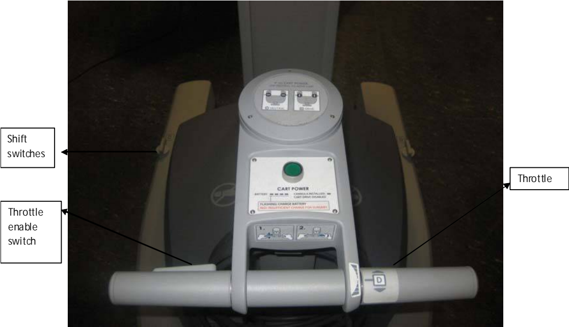
Fig. 2: Location of Throttle, Throttle Enable Switch, and Shift Switches
