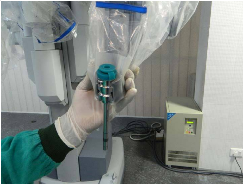
Fig. 20: Example of mounting instrument arm on to the cannula
