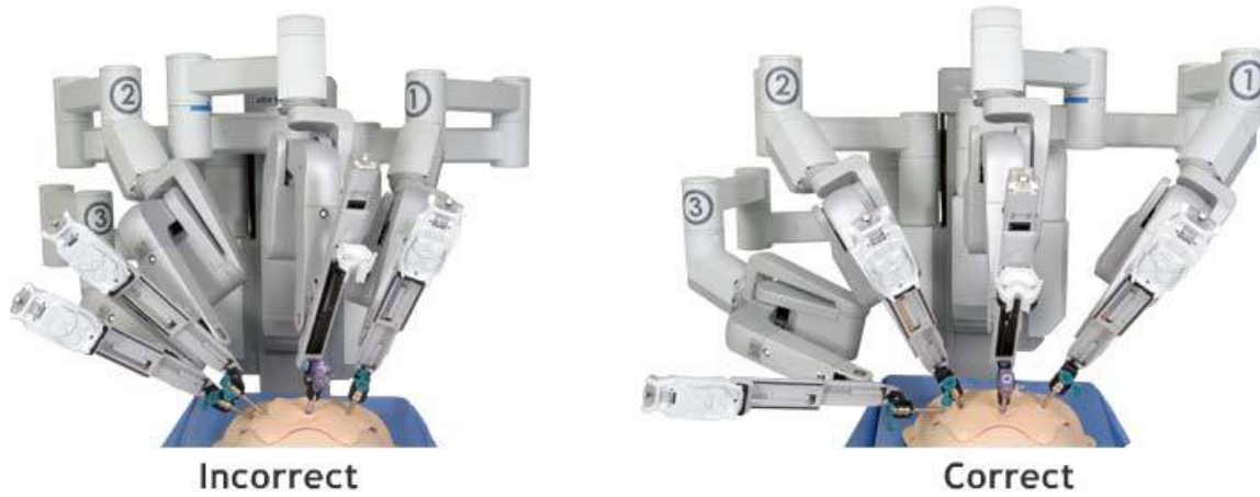
Fig. 23: Depiction of the correct method of docking of patient cart
