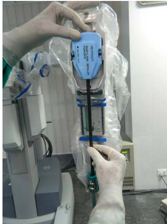
Fig. 27: Sliding the instrument into sterile adaptor on the instrument arm
