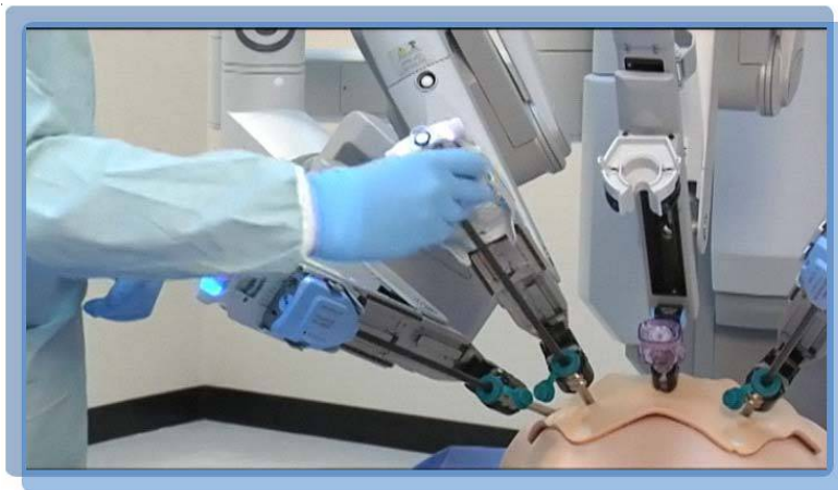
Fig. 30: Pressing the levers to remove the instrument
