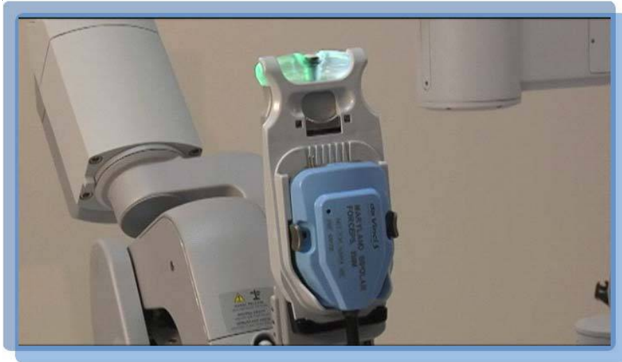
Fig. 31: LED blinking alternately white and green indicating activation of Guided Tool Change
