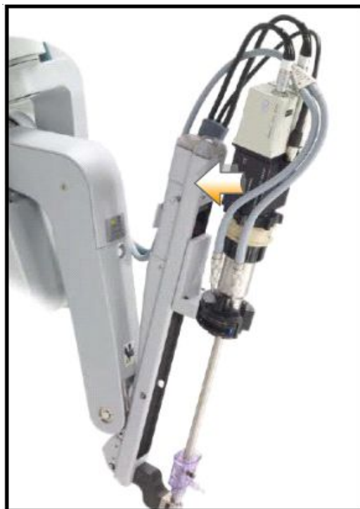
Fig. 24: Endoscope insertion into camera arm sterile adaptor of the camera arm
