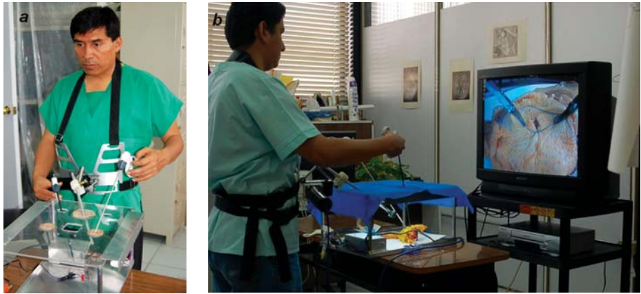
Figure 2. (a) From the design concept to the physical model, (b) hand – eye adaptation in training boxes suturing chicken pieces.
